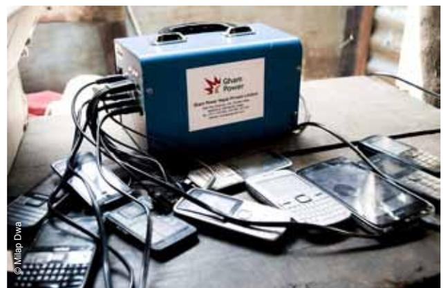
*Solar power units, such as this one charging 10 phones simultaneously, contributed to ensure communications in critically hit remote communities were maintained.*
