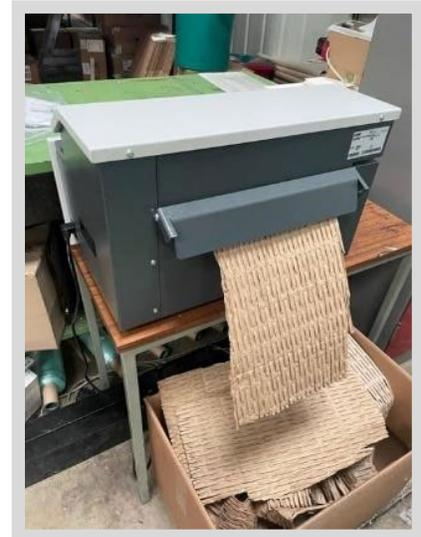
Figure 14: Cardboard boxes are shredded and used as infill for air freight.
