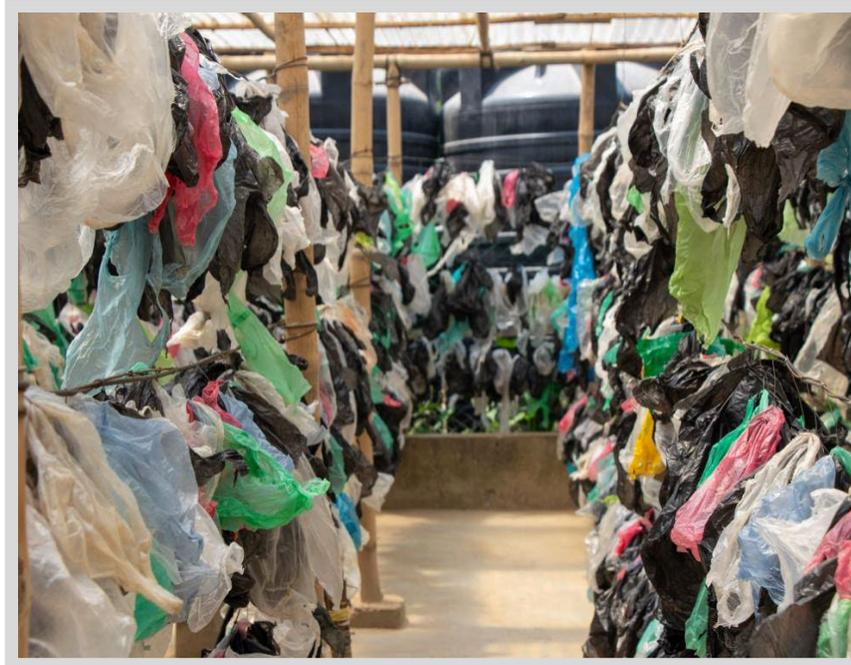
Figure 5: A view of the drying unit where washed plastic waste is kept for drying and then recycled into various useful objects. Photo: IOM/Tarek Mahmud.
