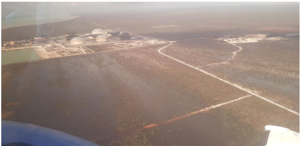
Figure 3: Aerial assessment of the facility, showing the plume of oil along the northeast direction as well as flooding on the East side of the plant (© PAHO)
