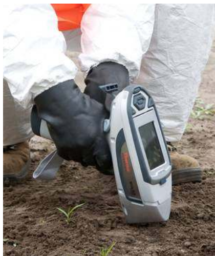
Figure VIII: Lead measurements were taken on location with the X-Ray Fluorescence analyser (XRF). The apparatus gives direct readings without taking samples.
