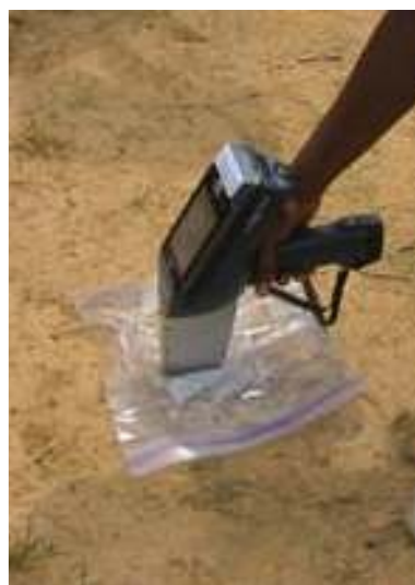
Figure IV: The X-Ray Fluorescence analyser (XRF) used as a lead screening device. The XRF gave an indication of the lead content in top soil and wet sediment.
