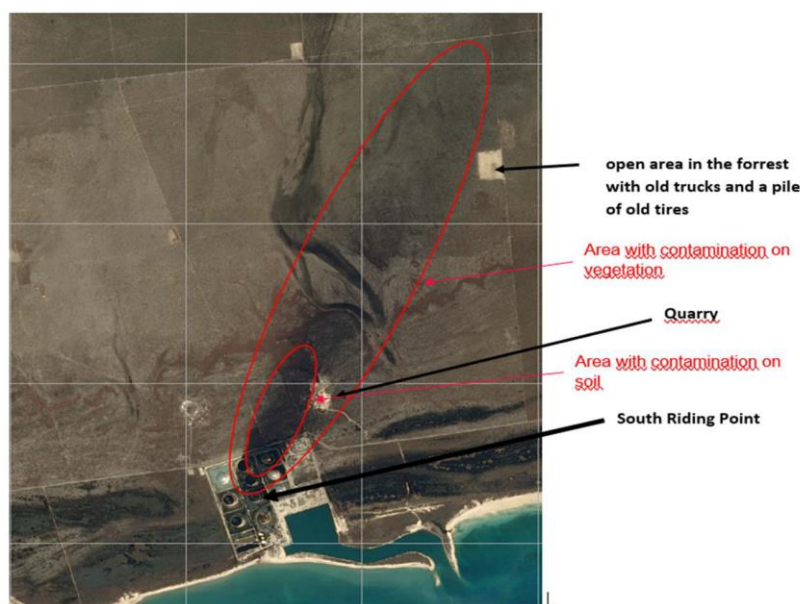
Figure 4: Extent of oil contamination inland (© Equinor)
